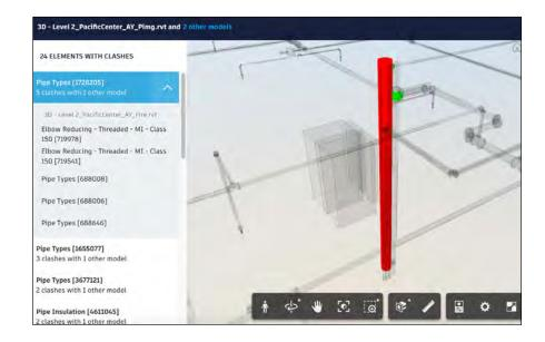
PRO TIP: Search and filter models within the clash matrix (using model naming conventions) to focus review on a specific location. Click on the row header to open and view all models and clashes within that context.
