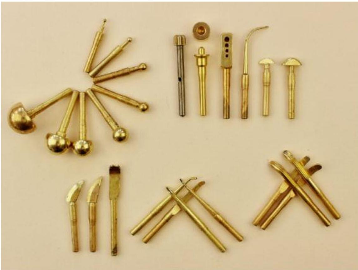
These days an electric soldering iron fitted with special flower making interchangeable heads is used to texture and shape petals and leaves.
